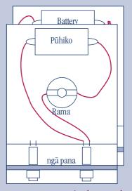
wired correctly battery, light and one switch in service
